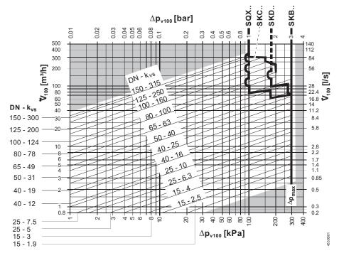
Δp<sub>max</sub> = Maximum permissible differential pressure across the valve (mixing: port A-AB, B-AB; diverting: port AB-A, AB-B), valid for the entire actuating range of the motorised valve
