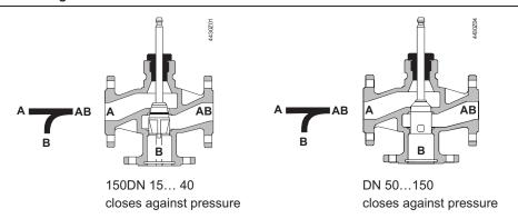
Guided plug which is integrated in the valve stem. The seats are machined in the valve body. Schematic representation, design variations are possible.
