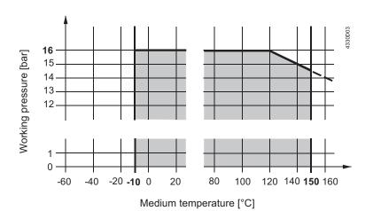
Working pressure and medium temperature staged as per ISO 7005
