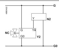
Y Positioning signal DC 0...10 V
