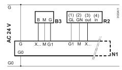
Diagram 5: Connection of a 2-speed fan
