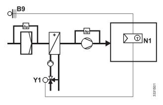
Room temperature control through control of the heating valve, with outside temperature compensation
