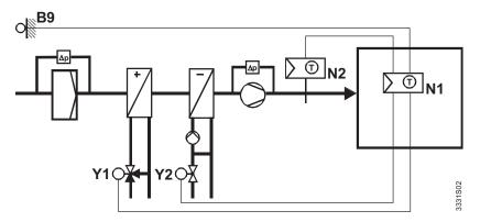
Room temperature control through control of the heating and cooling valve, with outside temperature compensation and limitation of the supply air temperature
