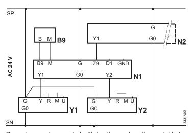
Room temperature control with heating and cooling, outside temperature compensation and minimum limitation of the supply air temperature
