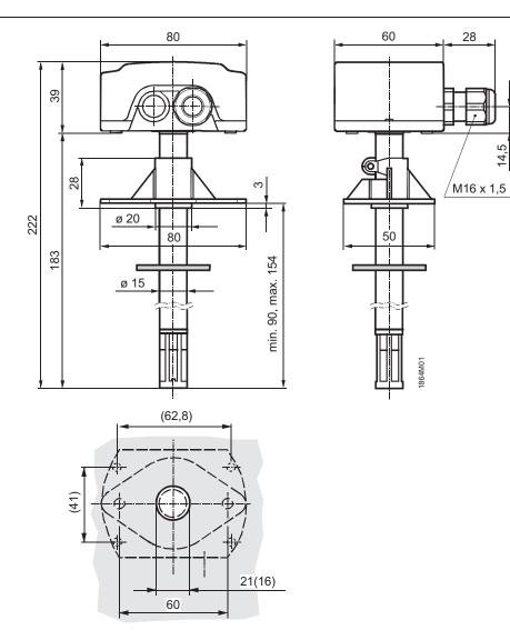
Drilling plan with (without) mounting flange
