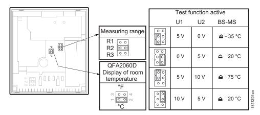
The setting elements are located in the casing. A setting element consists of 6 pins and a jumper. It is used for selecting the required temperature measuring range and for activating the test function. Types with LCD display have a second setting element with 4 pins and a jumper.
